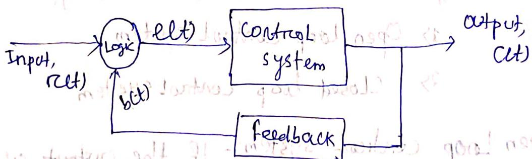
$b(t)$  → base signal / feedback signal
