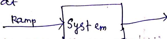
$$IR = \frac{d}{dt} \left\{ \begin{array}{l} \text{Step response} \\ \text{of } (1) \end{array} \right\} - (2)X$$
